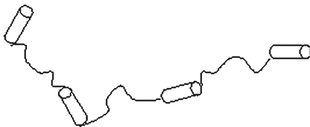
FIGURE 1 Main-chain nematic polymer. Cylinders represent the nematogenic units, and curved lines stand for the flexible parts of the chains.
